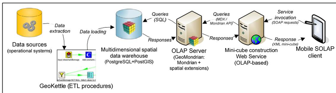
Fig. 3. Architecture of the Web service for SOLAP mini-cube delivery [17]
