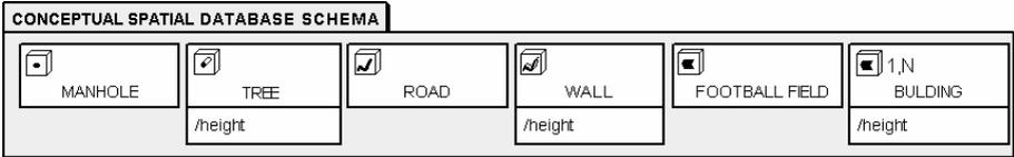
Fig. 3. Subset of a conceptual 3D data schema (not involving associations and methods)
